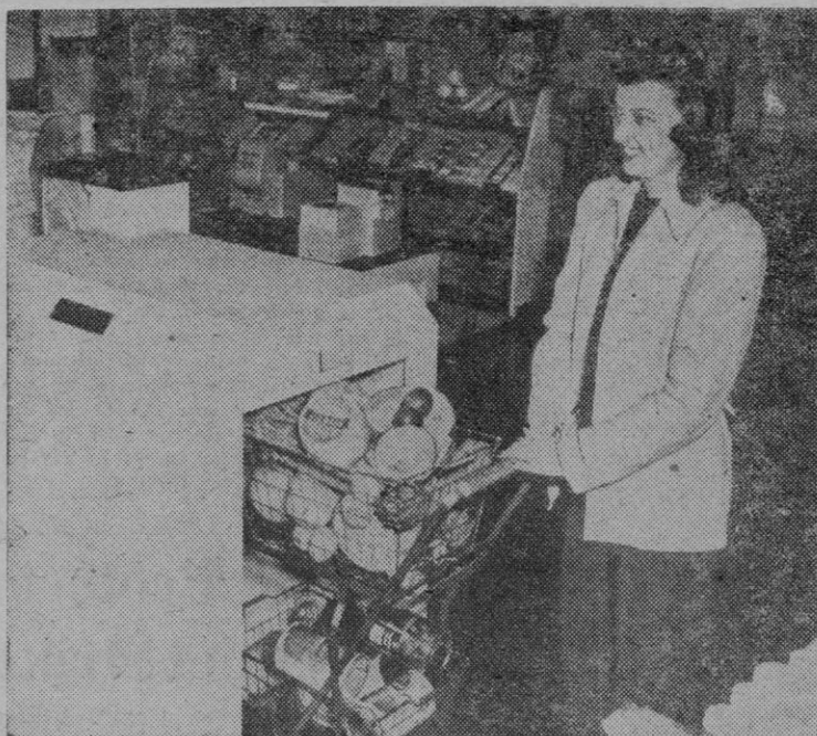
GERM EXTERMINATOR: Grocery baskets are passed through this device, which contains ultra-violet lamps, and are freed from germs. It is an innovation of a market in Spokane, Wash.
