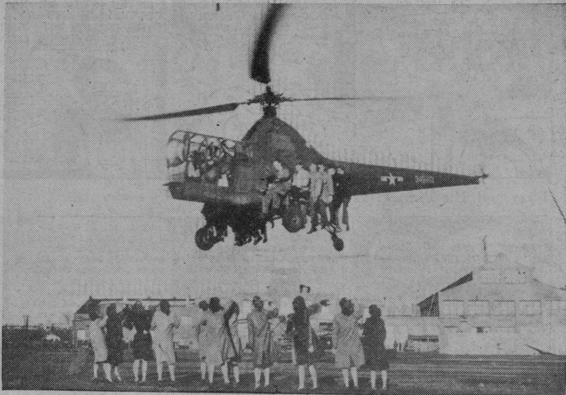
Here's the "family model" helicopter, produced at Bridgeport, Conn. and known as the Army-Sikorsky R5. In its test flight, shown above, it carried 18 men, who swarmed over the little plane and hung on anywhere they could get a grip.
