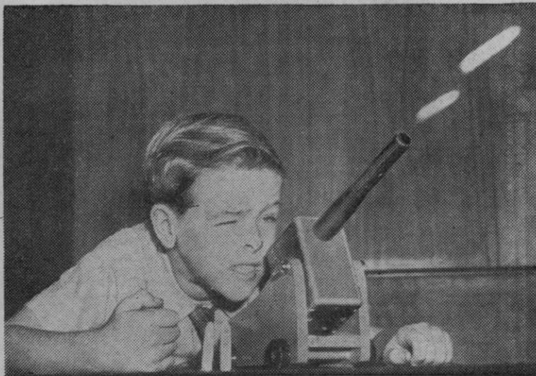
Ready to bombard toy soldiers is this electric cannon developed by the Elec-Toy Co. of Indianapolis. The gun fires wooden "shells" which are propelled by electro-magnetic force. The Nazis were using similar principles in construction of a new type of artillery weapon.
