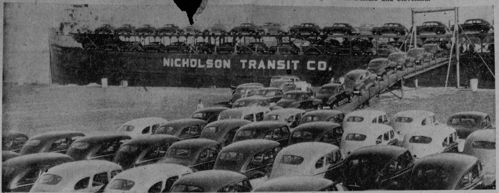
Carriers, fashioned with a deck similar to an aircraft carrier, are busy shuttling across the Great Lakes between Detroit and Eastern markets. New cars are shown being driven aboard the freighter for shipment to Buffalo and Cleveland.
