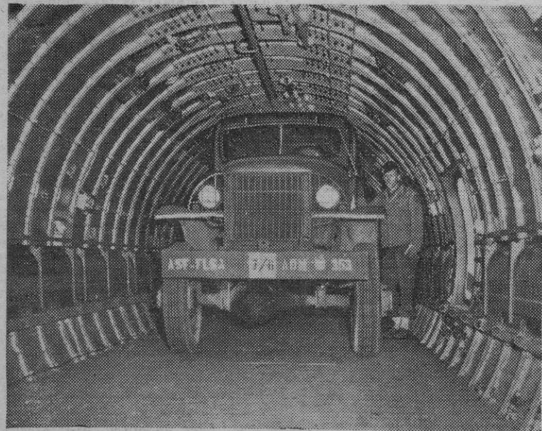
A 11/2-ton Army truck parked in the upper fuselage section of the new Boeing C97 air transport, which has a capacity like a boxcar. Two such trucks can ride on the main deck, with other equipment. Personnel or cargo may be carried in the two compartments of the lower deck. On its maiden delivery flight, the C97 sped nonstop from Seattle to Washington, D.C., in six hours and four minutes.
