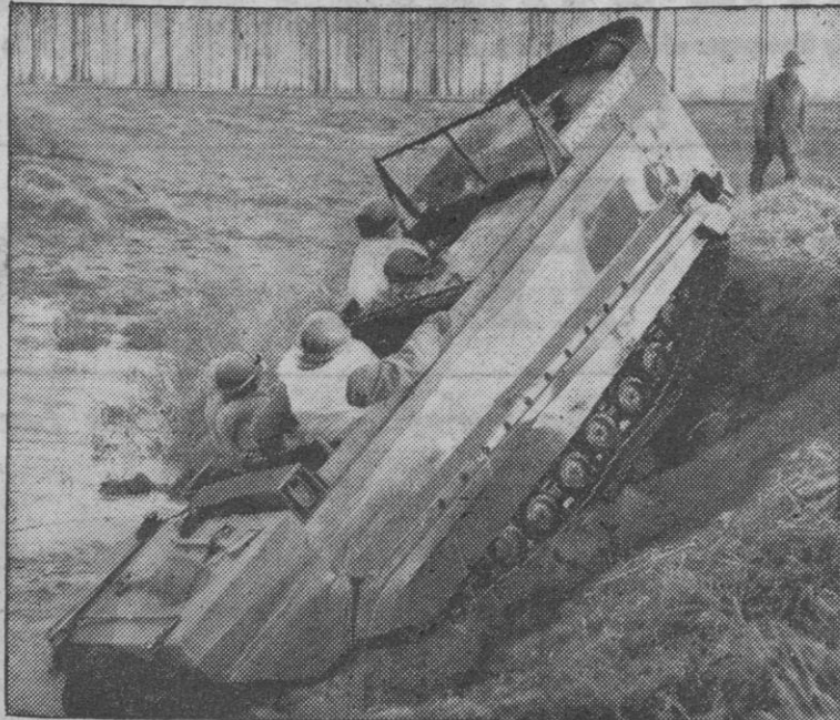
Climbing a steep bank after crossing a river is just one of the things the new "Weasel" can do. It is shown here during a test run in a training area behind the lines.
