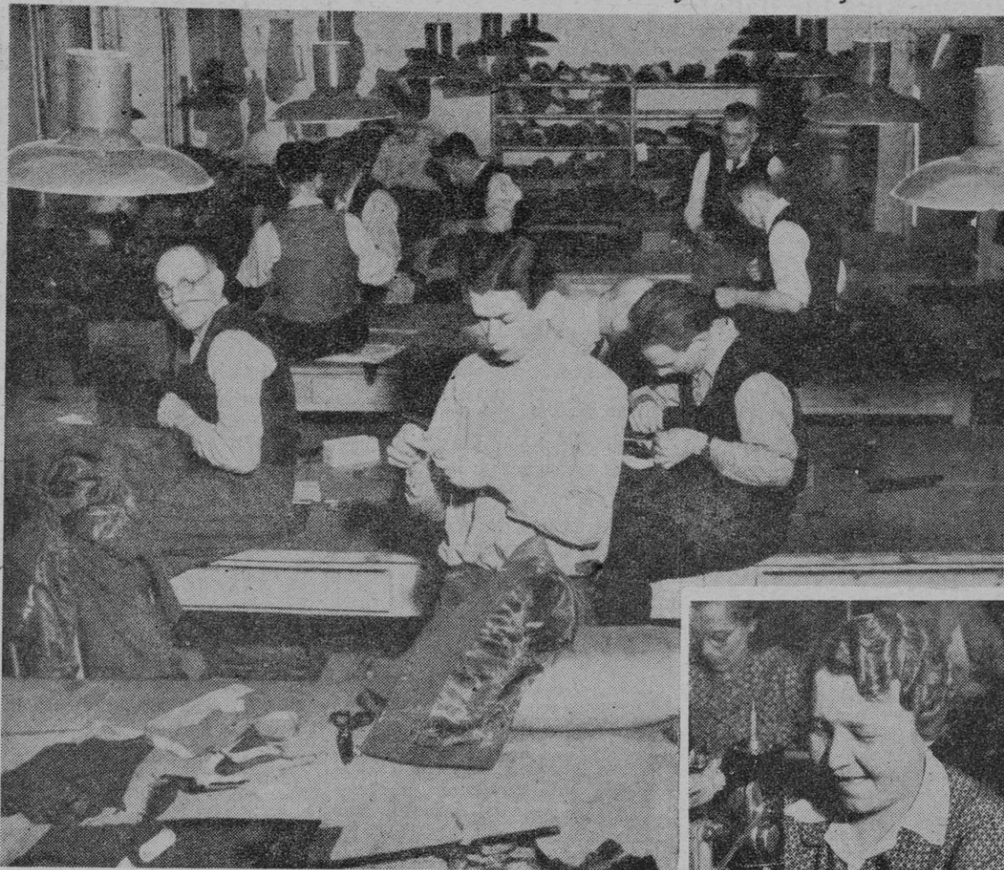
A COMPLETE CLOTHING FACTORY in Frankfurt, operated by Germans under U.S. Army supervision, is turning out general QM issue for European Theater troops. Civilian employes are shown at work in the factory's tailor shop. A woman operator (right) works on a machine which can cut and stitch 2,200 buttonholes an hour.
