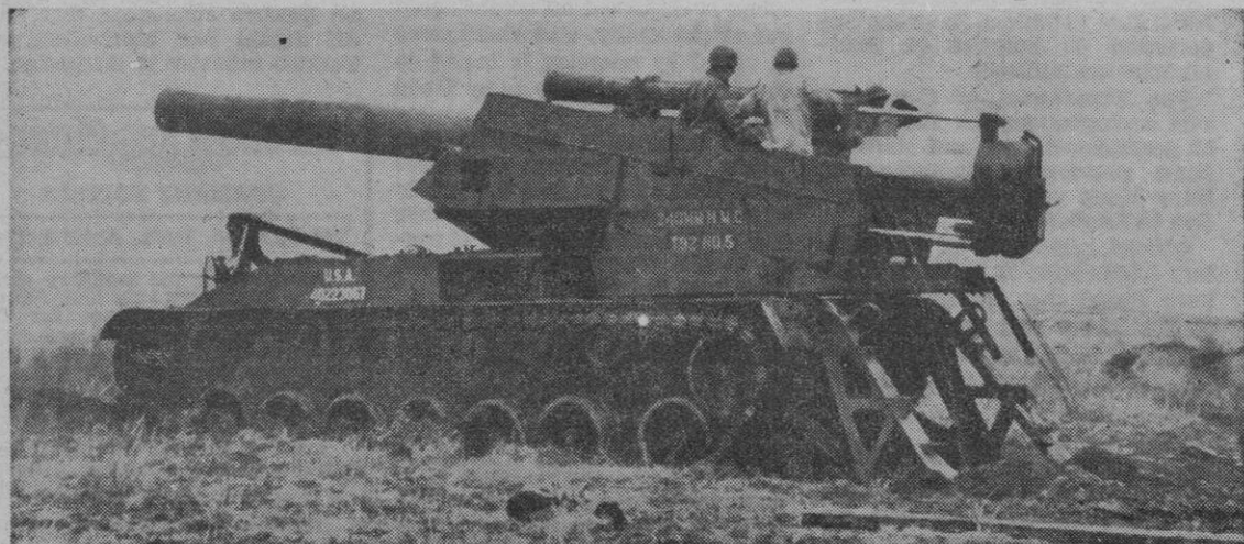
THIS GIANT HOWITZER, the "King Kong" of U. S. Army field artillery weapons, is seen in full recoil immediately after delivering one of its 350-pound shells at a testing ground at Ft. Sill, Okla. It is known as the 240-MM howitzer, is self-propelled and weighs 63 tons. —Acme Photo
