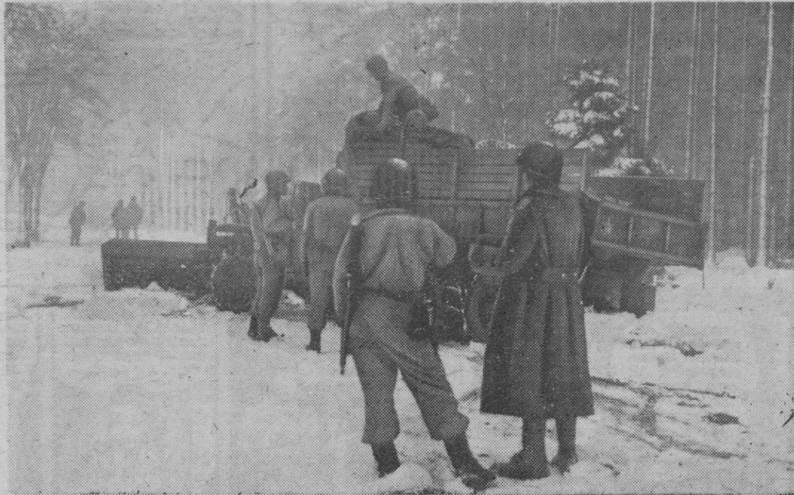
U.S. Army Signal Corps photo. Snow blocking a road near Krinkelter, Belgium, slowed down U.S. First Army movements, so engineers of the Second Inf. Div. rigged up this GI snow plow. A blade is mounted on a 2 1/2-ton truck.
