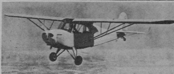
Already rolling off assembly lines, the Aeronca Champion, selling for $2,095, has a cruising speed of 90 MPH and lands at 35 MPH.
