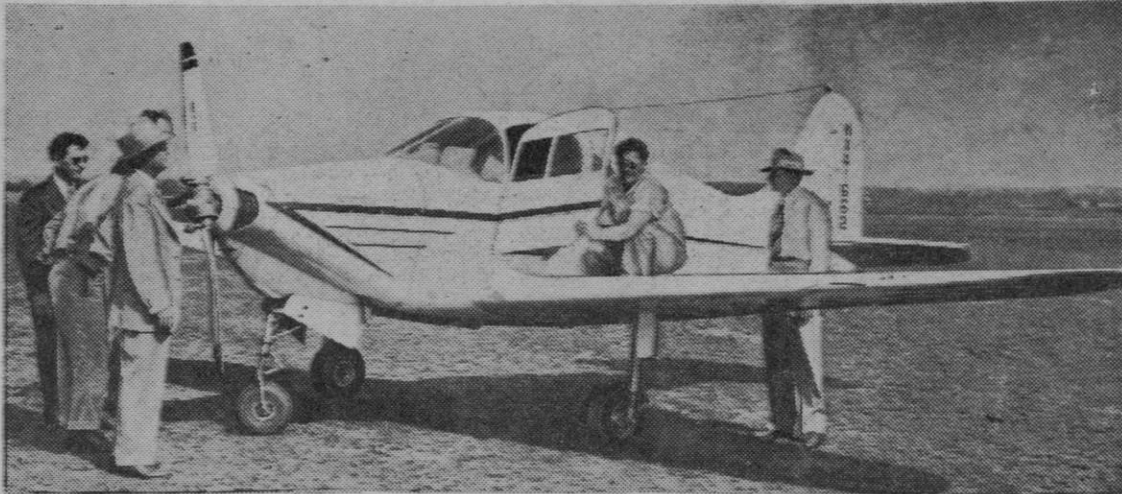
Makers say the new Rocket 185 will operate at a cost of one-half cent a passenger mile. The lightweight ship can cruise at 185 miles an hour and can climb 2,000 feet a minute.
