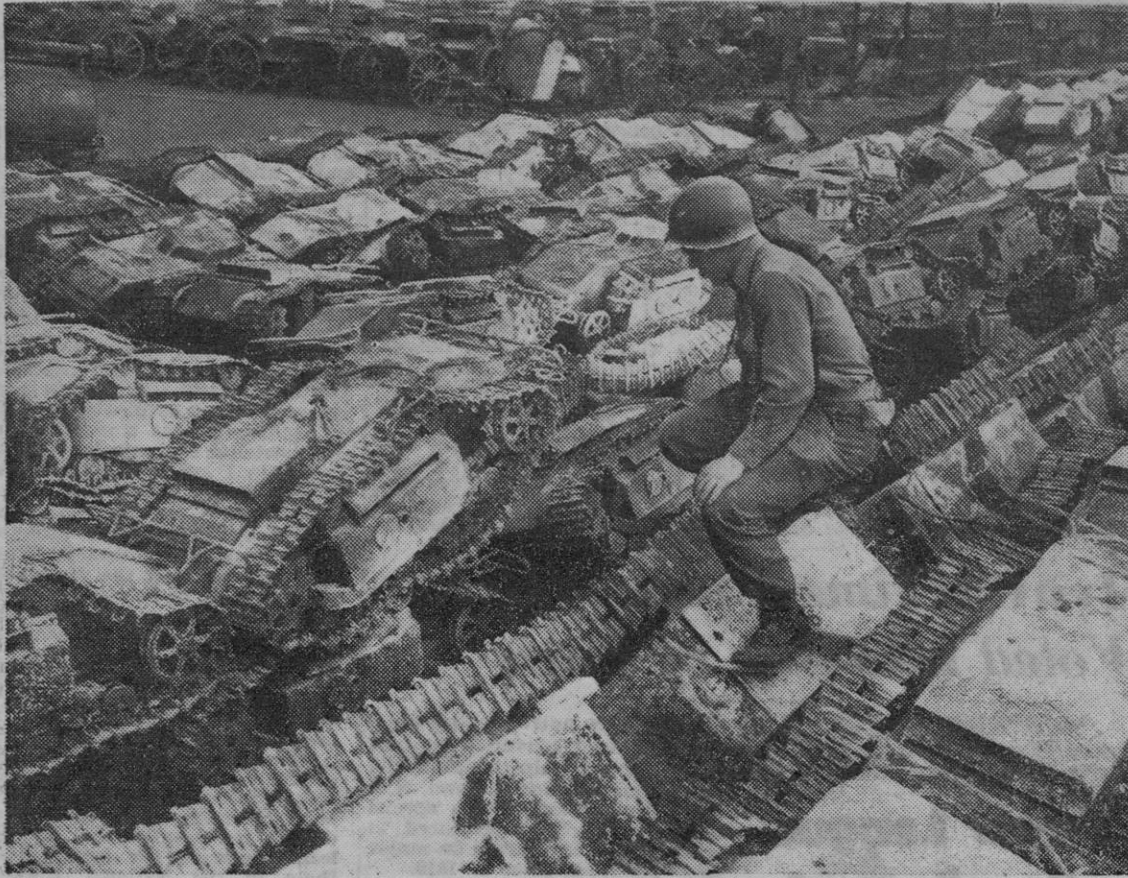
A soldier inspects rows of "doodle bugs," remote-control miniature tanks, captured when Bamberg fell to U.S. Seventh Army troops. The tanks, filled with explosive, are designed to be directed against strongpoints and blow up when they reach their destination.
